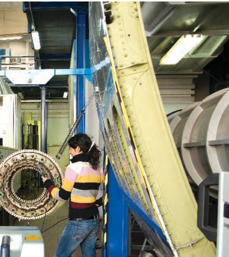
A Boeing-funded master's degree program at Italy's University of Naples Federico II is equipping students with systems engineering skills. Professor Leonardo Lecce (center) works with Igor Bovio (left) and Benedetta Capano in a lab where the students are using a scanning laser vibrometer to conduct experimental model analysis on an aircraft engine component.
